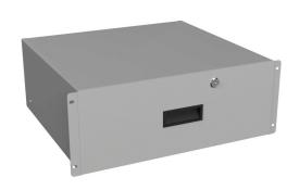
Hammond locking rack drawer, 4U, 19in rack width, 16.25in depth, carbon steel, RAL 7035 light gray, textured powder coat finish.
