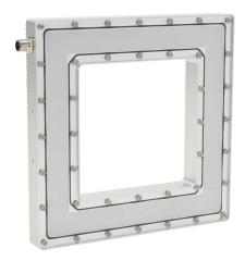
Lumher RD machine vision lighting, ring light, white light emission, 5000K, plus or minus 55 degrees, continuous and strobe, 225 x 225 x 25mm housing, 22.8-25.2 VDC operating voltage.
