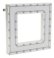
Lumher RD machine vision lighting, ring light, white light emission, 5000K, plus or minus 30 degrees, continuous and strobe, 225 x 225 x 25mm housing, 22.8-25.2 VDC operating voltage.
