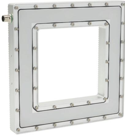
Lumher RD machine vision lighting, ring light, white light emission, 5000K, plus or minus 30 degrees, continuous, 225 x 225 x 25mm housing, 22.8-25.2 VDC operating voltage.
