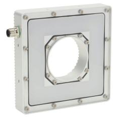
Lumher RD machine vision lighting, ring light, white light emission, 5000K, plus or minus 30 degrees, continuous and strobe, 135 x 135 x 25mm housing, 22.8-25.2 VDC operating voltage.
