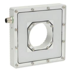
Lumher RD machine vision lighting, ring light, white light emission, 5000K, plus or minus 30 degrees, continuous, 135 x 135 x 25mm housing, 22.8-25.2 VDC operating voltage.
