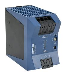
RECOM Power RACPRO1 series switching power supply, 24 VDC @ 40A/960W (adjustable), 480 VAC nominal input, 3-phase, enclosed, polycarbonate/aluminum housing, 4 segment load LED display, 35mm DIN rail mount, cage clamp.
