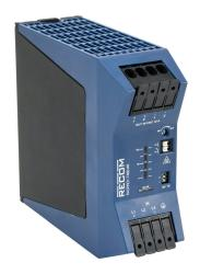
RECOM Power RACPRO1 series switching power supply, 48 VDC @ 10A/480W (adjustable), 480 VAC nominal input, 3-phase, enclosed, polycarbonate/aluminum housing, 4 segment load LED display, 35mm DIN rail mount, cage clamp.
