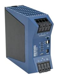
RECOM Power RACPRO1 series switching power supply, 24 VDC @ 20A/480W (adjustable), 480 VAC nominal input, 3-phase, enclosed, polycarbonate/aluminum housing, 4 segment load LED display, 35mm DIN rail mount, cage clamp.
