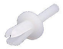
Iboco DUCTFIX expanding plastic rivet, natural. Package of 250. For use with Iboco duct and panel with a 0.26in (6.5mm) hole. Used with installation tool B6 for ease of use. Drill a hole sized 7/32in (5.5mm).
