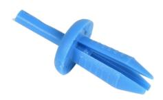
Iboco DUCTFIX expanding plastic rivet, blue. Package of 250. For use with Iboco duct and panel with a 0.17in (4.5mm) hole. Used with installation tool B4 for ease of use. Drill a hole sized 5/32in (4mm).
