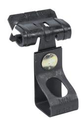
Minerallac side flange rod hanger, package of 25. For use with 1/8 to 1/4in side flange and 3/8-18 UNC threaded rod.
