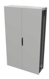
Quadritalia OKK series expansion bay kit, NEMA 12, 2000 x 1200 x 400mm (HxWxD), freestanding, carbon steel, RAL 7035 light gray, powder coat finish, double-door.
