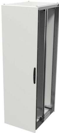
Quadritalia OKK series expansion bay kit, NEMA 12, 2000 x 600 x 800mm (HxWxD), freestanding, dual access, carbon steel, RAL 7035 light gray, powder coat finish, single-door.
