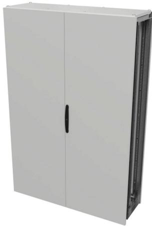
Quadritalia OKK series expansion bay kit, NEMA 12, 1800 x 1200 x 400mm (HxWxD), freestanding, dual access, carbon steel, RAL 7035 light gray, powder coat finish, double-door.
