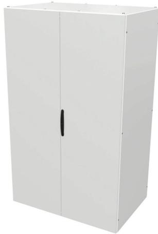
Quadritalia OKK series enclosure kit, NEMA 12, 2000 x 1200 x 800mm (HxWxD), freestanding, dual access, carbon steel, RAL 7035 light gray, powder coat finish, double-door.
