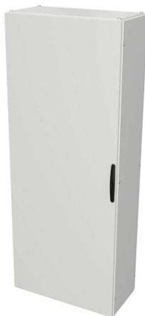
Quadritalia OKK series enclosure kit, NEMA 12, 2000 x 800 x 400mm (HxWxD), freestanding, dual access, carbon steel, RAL 7035 light gray, powder coat finish, single-door.
