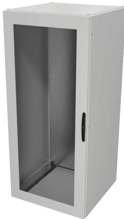
Quadritalia OKK series enclosure kit, NEMA 12, 1800 x 800 x 800mm (HxWxD), freestanding, carbon steel, RAL 7035 light gray, powder coat finish, single-door, acrylic window.
