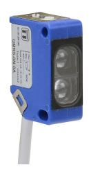
AutomationDirect photoelectric sensor, rectangular, plastic, diffuse with background suppression, 30-200mm sensing distance, selectable light-on/dark-on, NPN, potentiometer, 1 kHz switching frequency, 6.5ft/2m cable length, pigtail.
