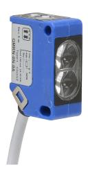
AutomationDirect photoelectric sensor, rectangular, polarized retroreflective, visible red, 0.1-5m sensing distance, selectable light-on/dark-on, NPN, potentiometer, 3-wire, pigtail.
