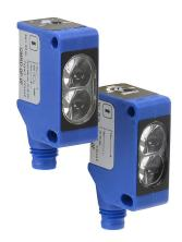
AutomationDirect photoelectric sensor, rectangular, plastic housing, through-beam pair, visible red, 0-20m sensing distance, 10-30 VDC operating voltage, selectable light-on/dark-on, PNP, 3-wire, 4-pin M8 quick-disconnect.
