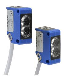
AutomationDirect photoelectric sensor, rectangular, plastic housing, through-beam pair, visible red, 0-20m sensing distance, 10-30 VDC operating voltage, selectable light-on/dark-on, PNP, 3-wire, pigtail.
