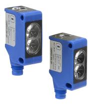
AutomationDirect photoelectric sensor, rectangular, plastic housing, through-beam pair, visible red, 0-20m sensing distance, 10-30 VDC operating voltage, selectable light-on/dark-on, NPN, 3-wire, 4-pin M8 quick-disconnect.
