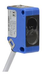
AutomationDirect photoelectric sensor, rectangular, retroreflective, visible red, 0.05-1m sensing distance, selectable light-on/dark-on, PNP, potentiometer, 3-wire, pigtail.
