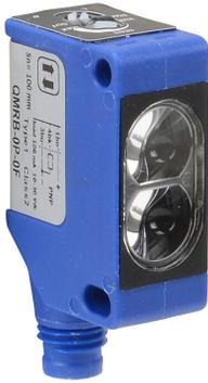
AutomationDirect photoelectric sensor, rectangular, diffuse, visible red, 5-100mm sensing distance, selectable light-on/dark-on, PNP, potentiometer, 1 kHz switching frequency, plastic housing, 4-pin M8 quick-disconnect.
