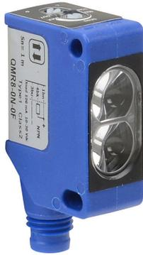
AutomationDirect photoelectric sensor, rectangular, diffuse, visible red light emission, 0-1m sensing distance, selectable light-on/dark-on, NPN, potentiometer, 1 kHz switching frequency, plastic housing, 4-pin M8 quick-disconnect.
