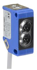
AutomationDirect photoelectric sensor, rectangular, diffuse, visible red, 0-400mm sensing distance, selectable light-on/darkon, PNP, potentiometer, 2 kHz switching frequency, plastic housing, pigtail.
