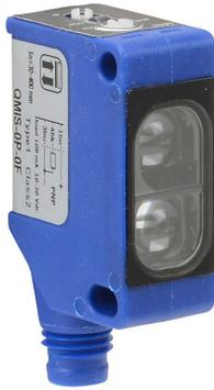
AutomationDirect photoelectric sensor, rectangular, plastic, diffuse with background suppression, 30-400mm sensing distance, selectable light-on/dark-on, PNP, potentiometer, 1 kHz switching frequency, 4-pin M8 quick-disconnect.
