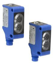
AutomationDirect photoelectric sensor, rectangular, plastic housing, through-beam pair, infrared, 0-30m sensing distance, 10-30 VDC operating voltage, selectable light-on/dark-on, PNP, 3-wire, 4-pin M8 quick-disconnect.
