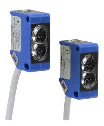
AutomationDirect photoelectric sensor, rectangular, plastic housing, through-beam pair, infrared, 0-30m sensing distance, 10-30 VDC operating voltage, selectable light-on/dark-on, PNP, 3-wire, pigtail.
