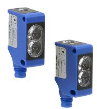
AutomationDirect photoelectric sensor, rectangular, plastic housing, through-beam pair, infrared, 0-30m sensing distance, 10-30 VDC operating voltage, selectable light-on/dark-on, NPN, 3-wire, 4-pin M8 quick-disconnect.
