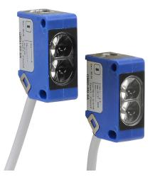
AutomationDirect photoelectric sensor, rectangular, plastic housing, through-beam pair, infrared, 0-30m sensing distance, 10-30 VDC operating voltage, selectable light-on/dark-on, NPN, 3-wire, pigtail.
