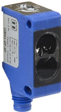
AutomationDirect photoelectric sensor, rectangular, retroreflective, infrared, 0.05-1m sensing distance, selectable light-on/dark-on, PNP, potentiometer, 3-wire, 4-pin M8 quick-disconnect.
