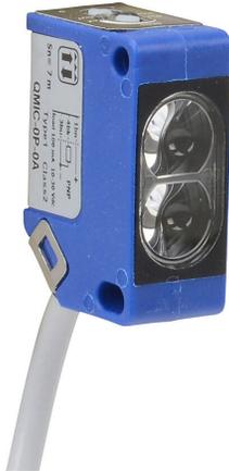
AutomationDirect photoelectric sensor, rectangular, retroreflective, infrared, 0.1-7m sensing distance, selectable light-on/dark-on, PNP, potentiometer, 3-wire, pigtail.
