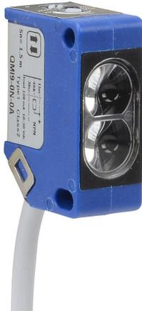
AutomationDirect photoelectric sensor, rectangular, diffuse, infrared light emission, 0-1.5m sensing distance, selectable light-on/dark-on, NPN, potentiometer, 1 kHz switching frequency, plastic housing, pigtail.
