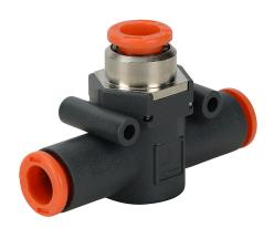
NITRA pneumatic push-to-connect fitting, inline quick exhaust valve, technopolymer body, 5/16in (8mm) tube inlet(s), 5/16in (8mm) tube exhaust(s).
