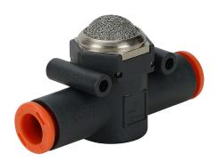
NITRA pneumatic push-to-connect fitting, inline quick exhaust valve, technopolymer body, (1) 5/16in (8mm) push-to-connect inlet(s), (1) 5/16in (8mm) push-to-connect outlet(s), (1) silenced exhaust(s).
