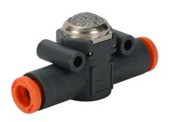
NITRA pneumatic push-to-connect fitting, inline quick exhaust valve, technopolymer body, (1) 1/4in push-to-connect inlet(s), (1) 1/4in push-to-connect outlet(s), (1) silenced exhaust(s).
