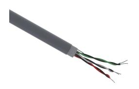
Quabbin RS-422 low capacitance data serial cable, shielded, 3 twisted pairs, 24 AWG, 7-stranded, tinned copper, polyethylene conductor insulation material, PVC jacket, gray, cut to length.
