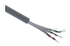
Quabbin RS-422 low capacitance data serial cable, shielded, 3 twisted pairs, 24 AWG, 7-stranded, tinned copper, foam polypropylene conductor insulation material, PVC jacket, gray, cut to length.
