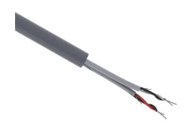
Quabbin RS-422 low capacitance data serial cable, shielded, 2 twisted pairs, 24 AWG, 7-stranded, tinned copper, foam polypropylene conductor insulation material, PVC jacket, gray, cut to length.
