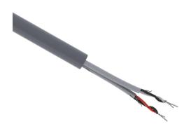
Quabbin RS-422 low capacitance data serial cable, shielded, 2 twisted pairs, 24 AWG, 7-stranded, tinned copper, foam polypropylene conductor insulation material, PVC jacket, gray, cut to length.
