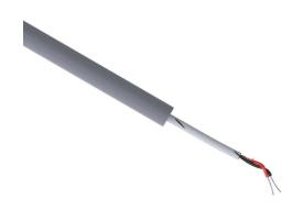
Quabbin RS-422 low capacitance data serial cable, shielded, 1 twisted pair, 24 AWG, 7-stranded, tinned copper, foam polypropylene conductor insulation material, PVC jacket, gray, cut to length.
