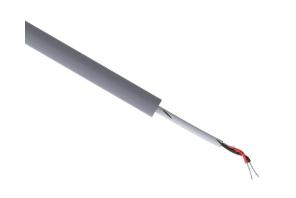
Quabbin RS-422 low capacitance data serial cable, shielded, 1 twisted pair, 24 AWG, 7-stranded, tinned copper, foam polypropylene conductor insulation material, PVC jacket, gray, cut to length.
