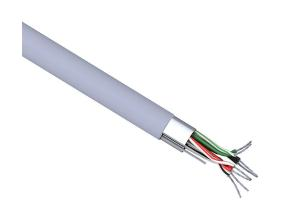
Quabbin control and signal cable, shielded, 4 twisted pairs, 24 AWG, 7-stranded, tinned copper, PVC conductor insulation material, PVC jacket, gray, cut to length.
