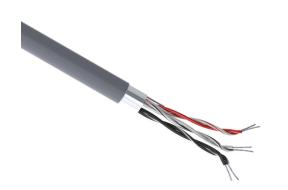
Quabbin RS-232 low capacitance data serial cable, shielded, 3 twisted pairs, 24 AWG, 7-stranded, tinned copper, PVC conductor insulation material, PVC jacket, gray, cut to length.
