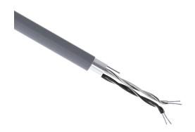
Quabbin RS-232 low capacitance data serial cable, shielded, 2 twisted pairs, 24 AWG, 7-stranded, tinned copper, PVC conductor insulation material, PVC jacket, gray, cut to length.
