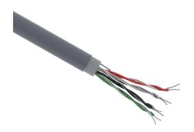
Quabbin RS-485 low capacitance data serial cable, shielded, 4 twisted pairs, 24 AWG, 7-stranded, tinned copper, polyethylene conductor insulation material, PVC jacket, gray, cut to length.
