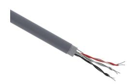
Quabbin RS-485 low capacitance data serial cable, shielded, 3 twisted pairs, 24 AWG, 7-stranded, tinned copper, polyethylene conductor insulation material, PVC jacket, gray, cut to length.
