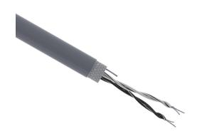
Quabbin RS-422/RS-485 low capacitance data serial cable, shielded, 2 twisted pairs, 24 AWG, 7-stranded, tinned copper, polyethylene conductor insulation material, PVC jacket, gray, cut to length.
