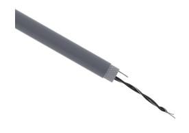
Quabbin RS-422/RS-485 low capacitance data serial cable, shielded, 1 twisted pair, 24 AWG, 7-stranded, tinned copper, polyethylene conductor insulation material, PVC jacket, gray, cut to length.
