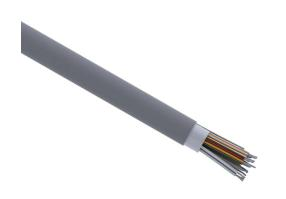
Quabbin control and signal cable, shielded, 25 conductors, 24 AWG, 7-stranded, tinned copper, PVC conductor insulation material, PVC jacket, gray, cut to length.
