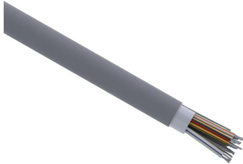
Quabbin control and signal cable, shielded, 25 conductors, 24 AWG, 7-stranded, tinned copper, PVC conductor insulation material, PVC jacket, gray, cut to length.
